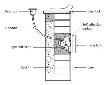
Note When installing an underwater light it is recommended the gland on the back of the light niche is checked and tightened to avoid water leaks.
