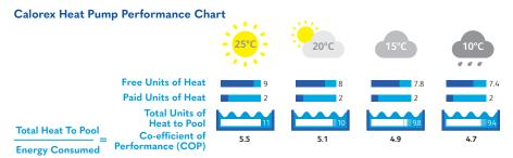
Sunshine is not essential for this system as all it needs is air; A heat pump can work with air temperatures as low as -15°C (dependent on the model chosen) and then becomes more efficient as the air temperature increases.
