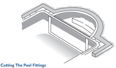
Gaskets should be applied to the surface all pool shell fittings prior to beginning the liner installation. The pool fittings should not be cut until the water level is immediately below the fitting.
