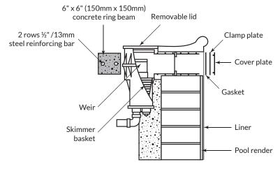
The surface skimmer has two functions. It removes surface debris, flies etc., from the pool surface and is also used as the vacuum point for attaching the vacuum kit for cleaning the bottom of the pool.
